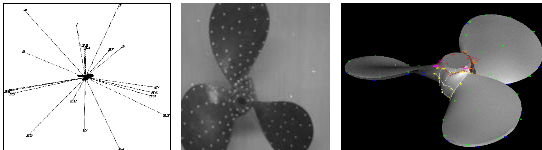
Fig. 7 (a) Nineteen camera stations (b) A View of Targets (c) Reconstructed CAD Model
