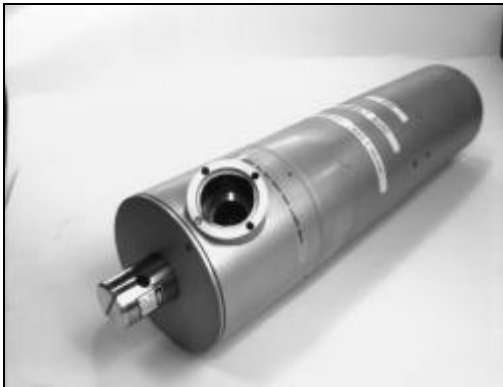
Fig. 4 (a) Pipe Profiling Instrument
