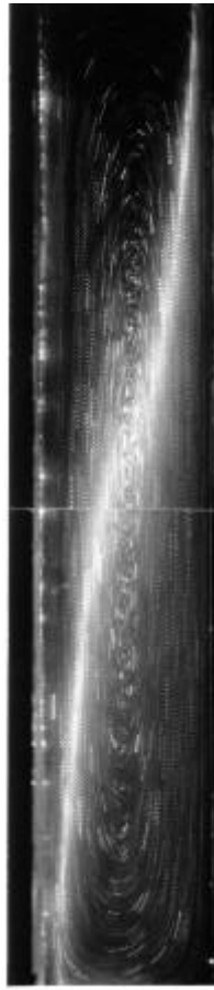
FIGURE 1. TEMPERATURE AND VELOCITY VISUALISATION IN GLYCEROL-FILLED CAVITY UNDER FREE CONVECTION USING TLC - VERTICAL POSITION. Ra = 1.2 \times 10^4 , Pr = 12.5 \times 10^3 , \Delta T = 10K .
