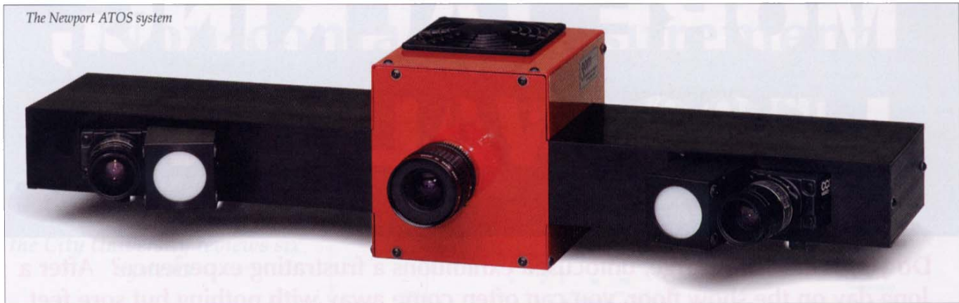
The Newport ATOS system An example of the matching of an appropriate system to a particular task is the use of the Newport ATOS system which uses two photogrammetric techniques to produce a high density surface information
