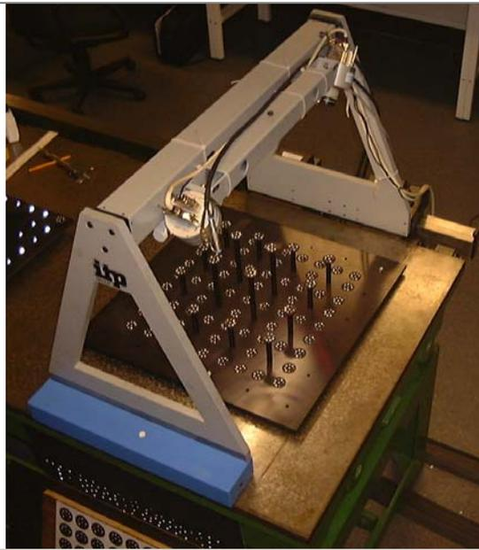
Calibration of the stereo head is achieved by using a calibration artefact. This procedure is only required on an irregular basis if the system tests show that a new calibration is required.
