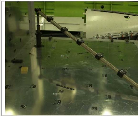
The OMC Quick Check method is suitable for quickly assessing a system. A rigid and lightweight artefact with a low expansivity co-efficient is used. The artefact is moved into a variety of locations as in the case of the full verification. However, in this case, the distance between the targets on the artefact is unknown. The average length between the targets is then estimated from all of the measurements and the rest of the measurements are compared to this average.
