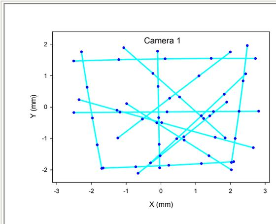
The resulting locations of the 3-D artefact in the image are given for one of the cameras in this figure. A good distribution of measurement positions in the image was tested.
