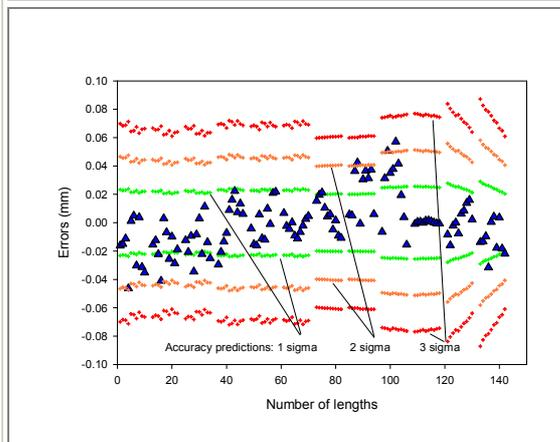
The accuracy of the stereo system in measuring the virtual length artefact was compared with the known lengths to arrive at a comparison. If the required number of measurement is within the statistical bounds the system passes the verification test.
