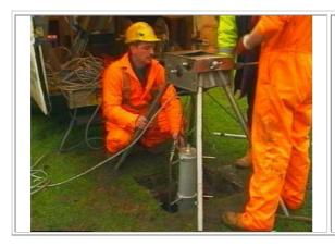
The Thames Water version of the profiler built upon experience developing and testing a previous prototype for North West Water. This device was able to measure 400 points in few seconds and function up to 95 metres from the operator.
