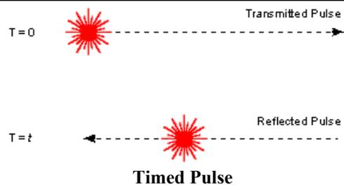
A short pulse of laser light is emitted, and the delay until its reflection returns is timed very accurately. If the speed of light is known, the distance to the reflecting object can be calculated. A single timed pulse is not very accurate, so a large number of pulses are used and averaged to give a more accurate distance. Hence there is a trade off between the accuracy and speed of measurement.
