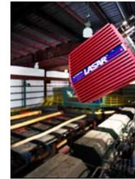
*Time-of-flight systems measure the time for a pulse of light to travel to a surface and return, then calculate distance from the constant speed of light*
